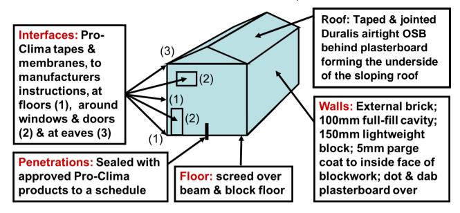
A more general additional statement for inclusion in any project specification might be: "All building elements and specialist components (such as curtain walling, roller-shutter doors, dock levellers etc.) must have a proven air leakage rate that is no more than 50% of the specified air-tightness for the whole building."
