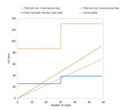
FIGURE 1. COMPARISON OF FLUSH PER USE AND TIMED FLUSH. CONSERVING WATER IN BUILDINGS, EA 2007.
