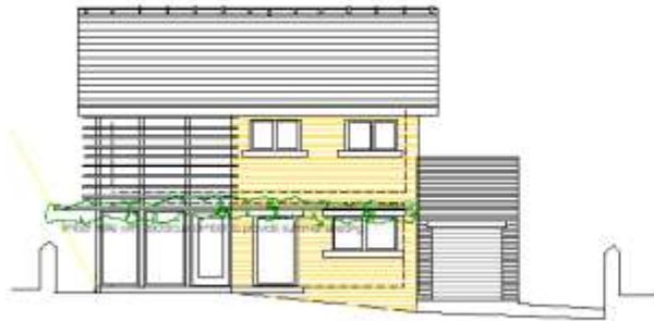
ELEVATION TO ACCESS ROAD ( south ) 1:100 in A3/LA
