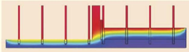
this cool structure from interstitial condensation – but might it worsen the risk from moisture from outside condensing there and damaging the timber? (See discussion in text of main article). One option that is sometimes deployed is to take the joists out of the masonry and suspend them from joist hangers – quite a big job though! On the Georgian retrofit described on this page, a combination of hygroscopic insulation, injected boron gel, and monitoring, was used as an alternative.
