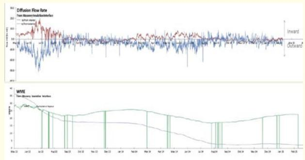
If you look at the net effect of both these lines (the blue line) it shows that it is always going down, or at worst level, which means overall, vapour is only being lost from the masonry, ie the newly refurbished building is drying out.
