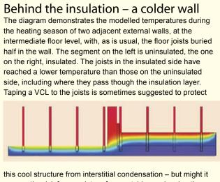
worsen the risk from moisture from outside condensation but high it and damaging the timber? (See discussion in text of main article). One option that is sometimes deployed is to take the joists out of the masonry and suspend them from joist hangers – quite a big job though! On the Georgian retrofit described on this page, a combination of hygroscopic insulation, injected boron gel, and monitoring, was used as an alternative.
