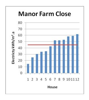
Again in square metre terms this looks high, but at 3600kWh/yr the average household consumption is 20% below the UK average. Comparisons were made between mechanical extract only ventilation, and heat recovery ventilation. Average heating
