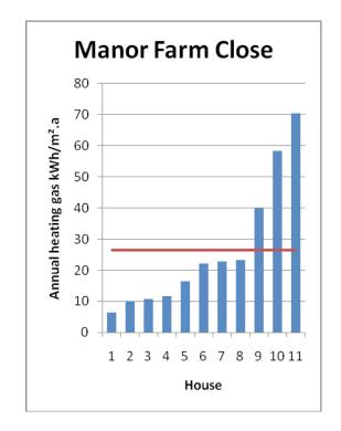
These results show the success in limiting building heat loss. The higher hot water energy consumption principally reflects the higher occupancy figures for these houses. These occupancy levels are typical for social housing, but unheard of in self-build "ecohouses". The high energy consumption for hot water despite best practice water efficient fittings informed the decision to install solar hot water on the third scheme.
