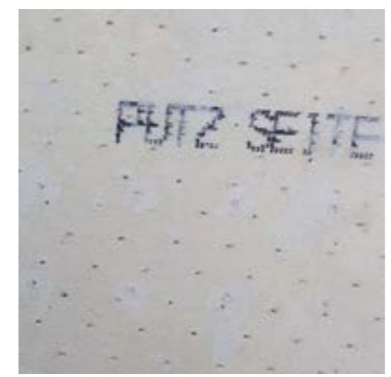
Name: Remmers iQ therm Material: PIR + capillary active plugs Location: internal wall insulation Thermal conductivity: 0.031 W/m.K Vapour diff resistance ( \mu ): 27
