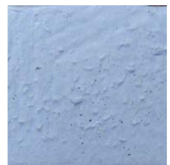
Name: Kingspan Styrozone N300R Material: extruded polystyrene Location: below ground external Thermal conductivity: 0.038 W/m.K Vapour diff resistance ( \mu ): high
