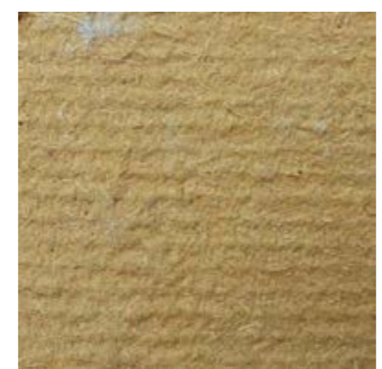
Name: Gutex Thermoroom Material: woodfibre Location: internal wall insulation Thermal conductivity: 0.04 W/m.K Vapour diff resistance ( \mu ): 3
