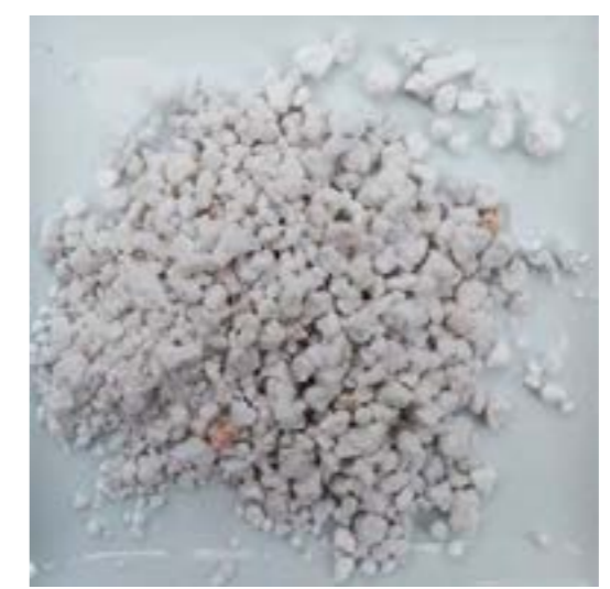
Name: Silvapor Material: perlite beads Location: stair stringer Thermal conductivity: 0.045 W/m.K Vapour diff resistance ( \mu ): low
