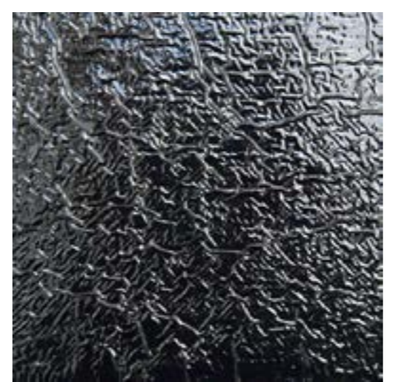
Name: Kevothermal VIP Material: vacuum insulated panel Location: ground floor below screed Thermal conductivity: 0.007 W/m.K Vapour diff resistance ( \mu ): \infty
