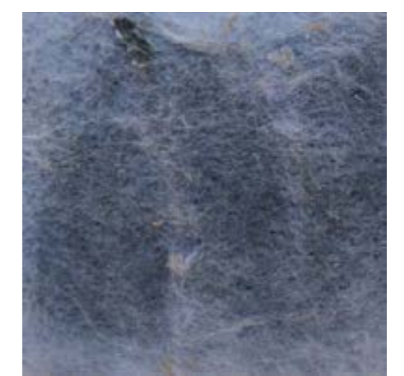
Name: Thermablok SP Material: aerogel blanket Location: internal wall insulation Thermal conductivity: 0.014 W/m.K Vapour diff resistance ( \mu ): 5.5
