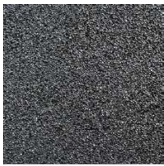
Name: Foamglas Perinsul Material: high density foamed glass Location: door and window sills Thermal conductivity: 0.058 W/m.K Vapour diff resistance ( \mu ): \infty
