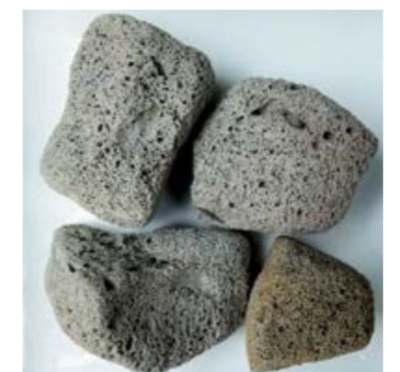
Name: Technopor Material: foamed glass granulate Location: external perimeter Thermal conductivity: 0.08 W/m.K Vapour diff resistance ( \mu ): low
