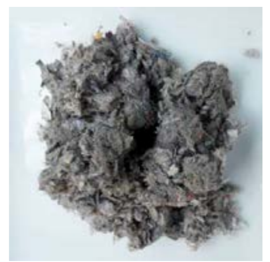
Name: Excel Warmcel 500 Material: blown cellulose Location: loft floor + shutter boxes Thermal conductivity: 0.04 W/m.K Vapour diff resistance ( \mu ): 2
