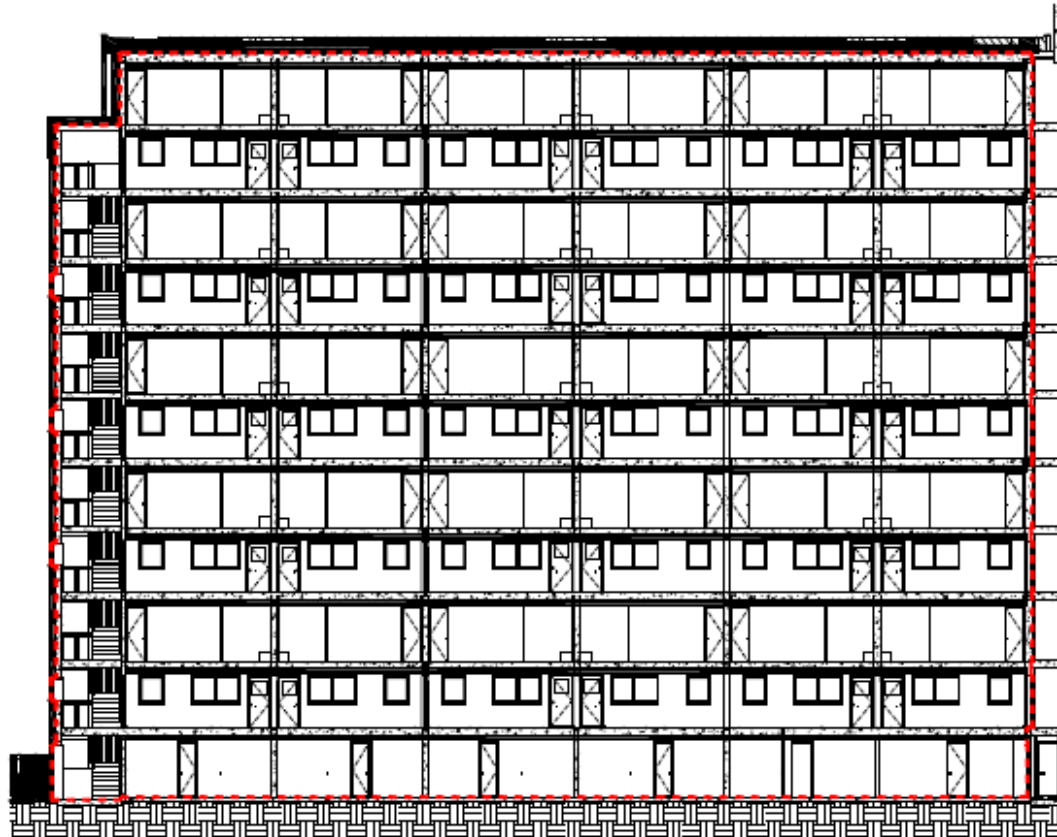
1 Typical Block Long Section - Air-tightness strategy 1:100
