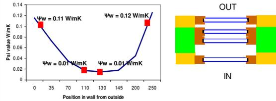
Schematic for illustration purposes based on installation positions for a high performance double glazed window into advanced specification cavity wall construction
