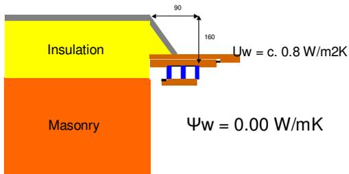
Schematic drawing based on an example from proceedings of the Passive House Conference 2006 for renovation of typical German construction using PH standard window. Freundorfer, Kaufmann and Krause
