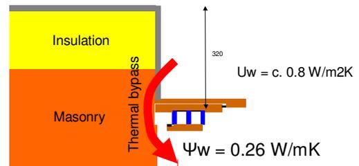
Schematic drawing based on an example from proceedings of the Passive House Conference 2006 for renovation of typical German construction using PH standard window. Freundorfer, Kaufmann and Krause
