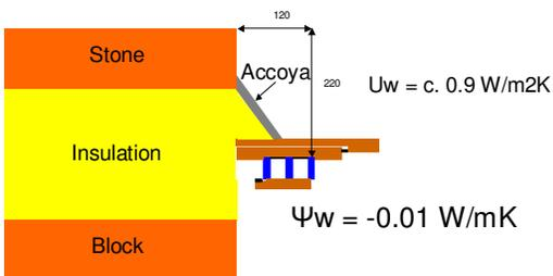
Schematic drawing based on cavity wall design for the Denby Dale House, courtesy Green Building Company
